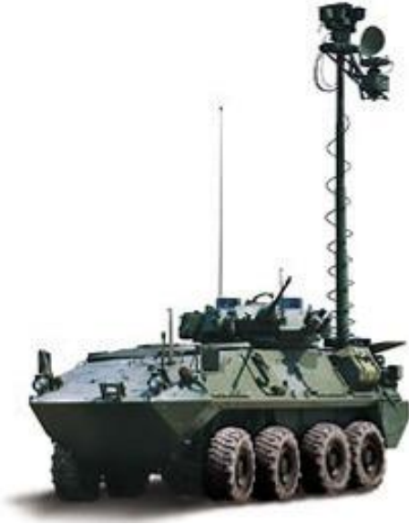
Figure 1: Coyote LAV with sensor mast deployed
